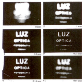
Figure: Historic pinhole cameras and tradeoff size of pinhole / sharpness.
