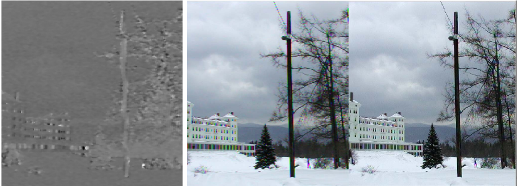
Figure: Median filtering, left: R-G signal, centre: bilinear interpolation, right: median filtering result
