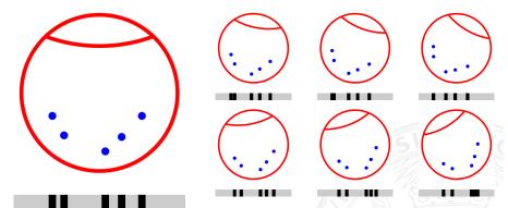
Figure: Longitudinal finger rotation principle: a schematic finger cross section showing five veins (blue dots) rotated from -10° to -30° (top row) and 10° to 30° (bottom row) in 10° steps. The projection of the vein pattern is different according to the rotation angle following a non-linear transformation.
