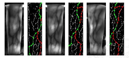
Figure: Examples of finger vein images and extracted MC features acquired at different longitudinal rotation angles. Left: -30°, middle: 0° (palmar view), right: 30°
