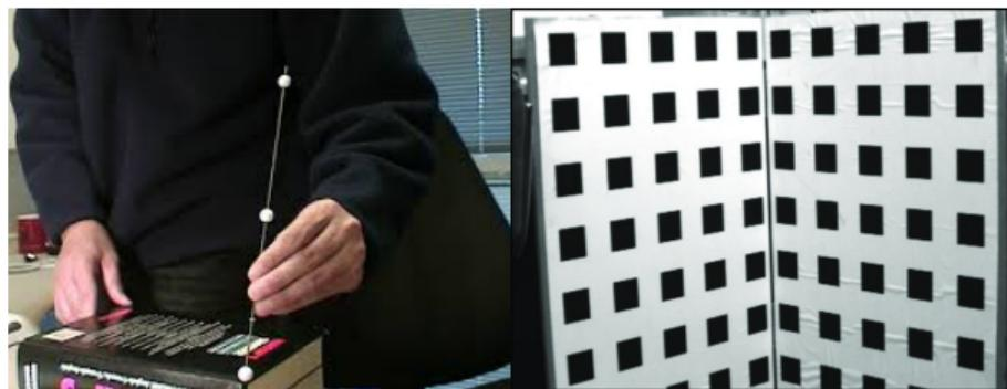
Bar with three collinear spherical objects as 1D calibration object (left) [Zhang, 2001] and spatial rectangular pattern (right) [Lioulemes, 2013].
