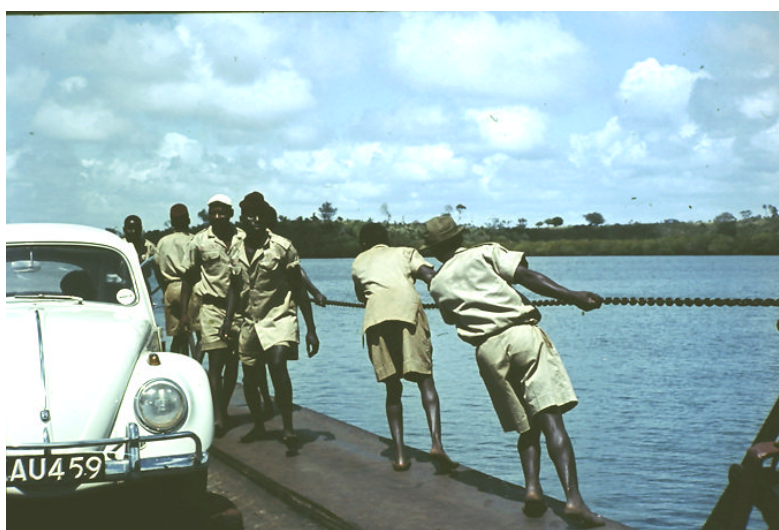
The ferryboat crosses Mtwapa Creek by man-power. The men pull on a chain spanning the creek.
