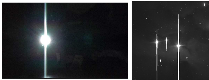
Figure 29: Smearing and blooming effects in CCDs configurations.
