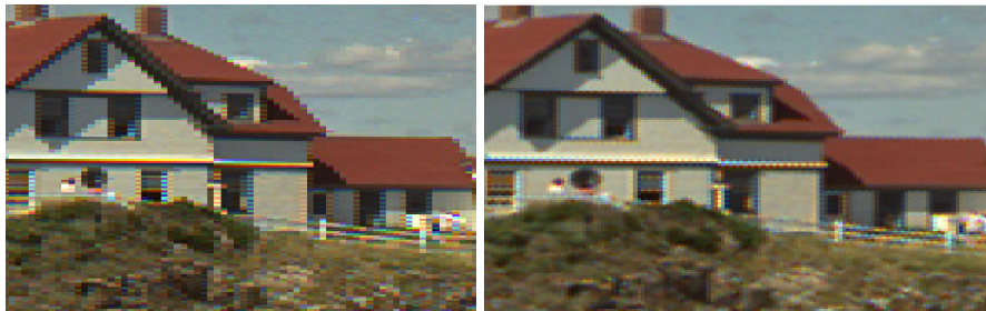
Figure 141: Examples for color plane interpolation: nearest neighbour vs. bilinear
