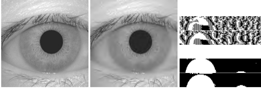
Fig. 3. Comparison of uncompressed/compressed iris image and the corresponding iris templates and noise masks
