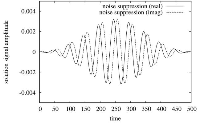
Fig. 4. Complex solution signal for artificial test set. The noise strength in comparison to signal strength is  $N = 20$ . The unmodified solution signal is too noisy to be shown in this plot.
