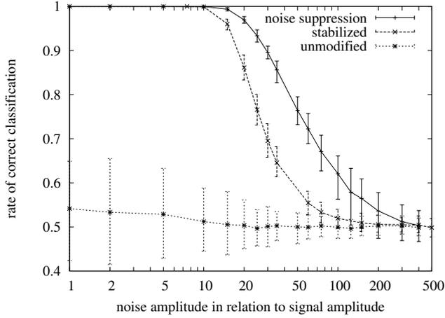
Fig. 3. Results of classification test for under-determined artificial test set depending on noise strength.
