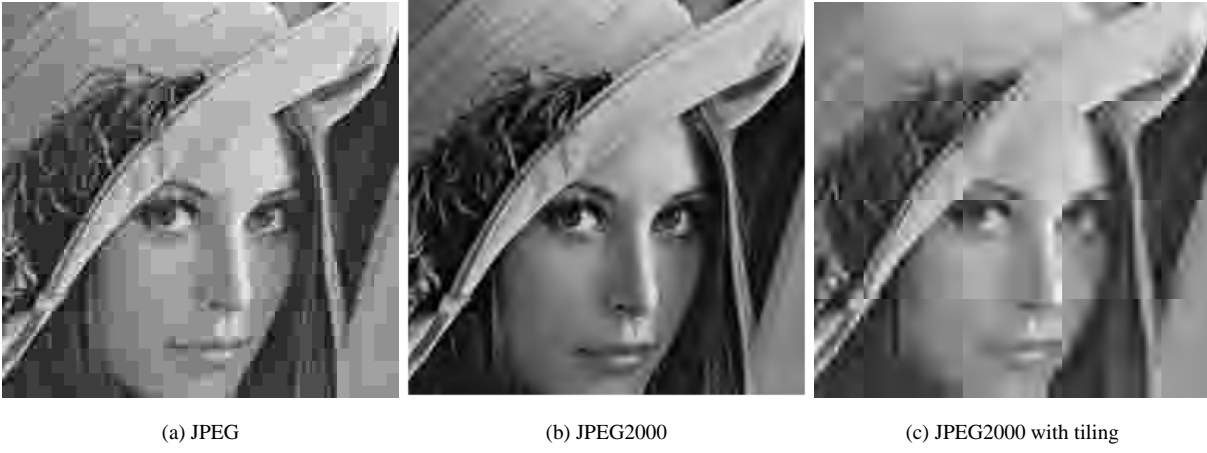
Figure 4. The center part of the Lena image coded with a bitrate of 0.125 bpp, on the left using JPEG, in the middle employing JPEG2000 without tiling, and on the right using JPEG2000 with a tile size of 64 \times 64 .
