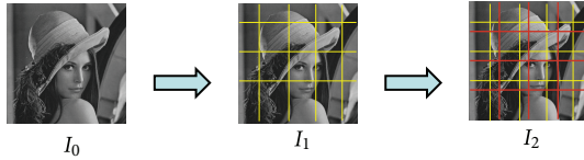
FIGURE 6: An example of nonaligned double JPEG (NA-DJPG) compression: the uncompressed image I_0 is first compressed, with a block grid shown in yellow, obtaining a single compressed image I_1 ; this image is again compressed, with a block grid shown in red, misaligned with the previous one, obtaining the final image I_2 .
