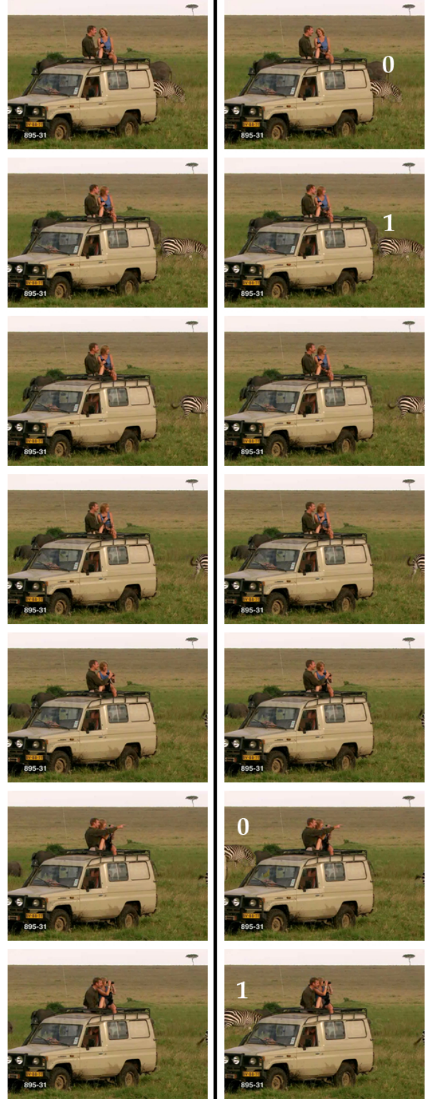
Figure 4: Shown in the left column are seven frames of an original video. Shown on the right are the results of region duplication so as to add another zebra into the scene.
