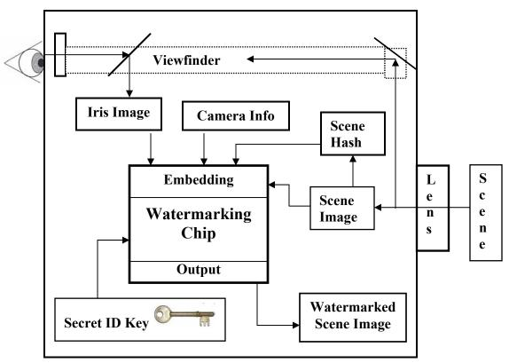
Figure 4. Secure Digital Camera (block diagram).
