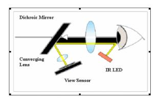
Figure 7. Canon eye controlled focus.
