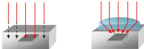
Figure 31: Microlens principle.
