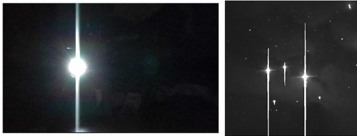
Figure 29: Smearing and blooming effects in CCDs configurations.
