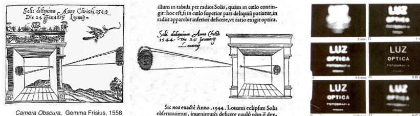
Figure 9: Historic pinhole cameras and tradeoff size of pinhole / sharpness.
