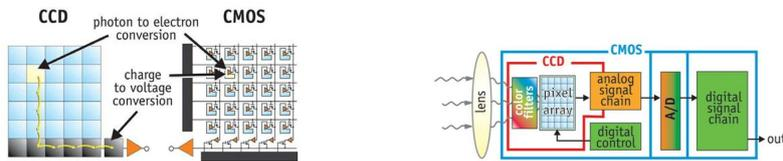
Figure 26: Schematic comparison of CCD and CMOS sensors.
