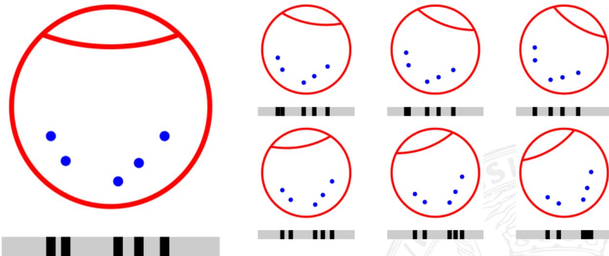
**Figure:** Longitudinal finger rotation principle: a schematic finger cross section showing five veins (blue dots) rotated from  $-10^\circ$  to  $-30^\circ$  (top row) and  $10^\circ$  to  $30^\circ$  (bottom row) in  $10^\circ$  steps. The projection of the vein pattern is different according to the rotation angle following a non-linear transformation.
