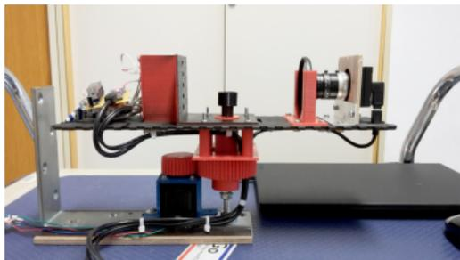
Figure: Custom build multi-perspective finger-vein scanner
