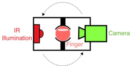
Figure: Basic principle of our rotating finger vein scanner
