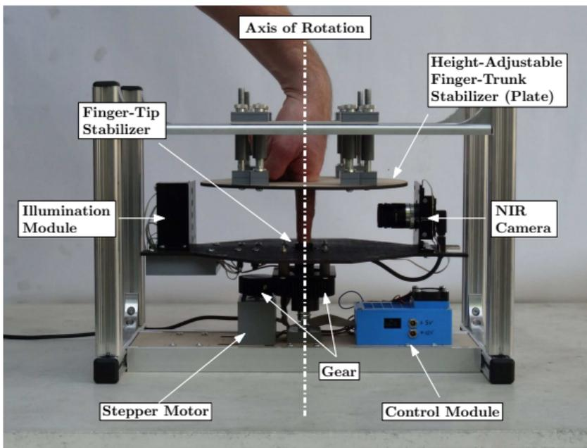
**Figure:** Multi-perspective finger vein scanner V2.0
